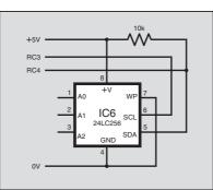
Fig. 10 Basic connections between a 24LC256 and a PIC16F877x.
