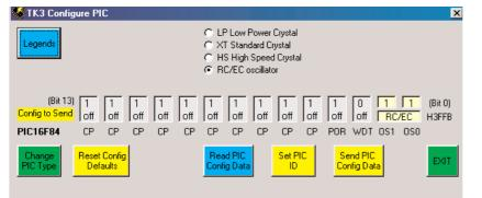
Configuration settings used for the first several experiments, putting the PIC16F84 into RC oscillator mode.
