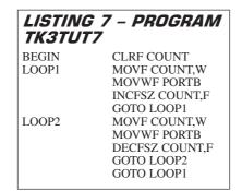
This represents the first example of the use of an "ordinary" file (as opposed to a Special Register File). Such files are used for temporarily storing data values while the program is being run. In the PIC16F84 the file addresses that can be used for this purpose are held in Bank 0 between H'OC' and H'2F'.
