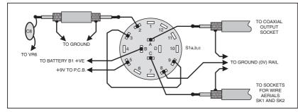
Fig.3. Wiring to the on/off and aerial selector switch. Pole letters and tag numbers match specified switch.
