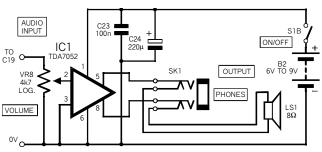
Fig 3. The audio power amplifier stage.
