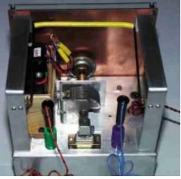
The chassis of the prototype was fabricated from aluminum and a wooden case with hinged lid holding the loudspeaker made to house the receiver. The lid can be raised and held up by a hinged wire frame (shown above) when in use.
