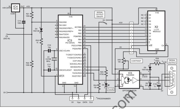
Fig.2. The Biopic's control circuit details.)
