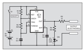
Fig.2. Circuit diagram for the original Zapper.
