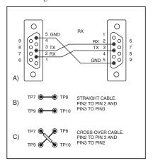
Fig.3. Links to be made in respect of serial lead type, see text.
