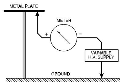
**Fig. 1. Basic principle of atmospheric electricity monitoring.**
