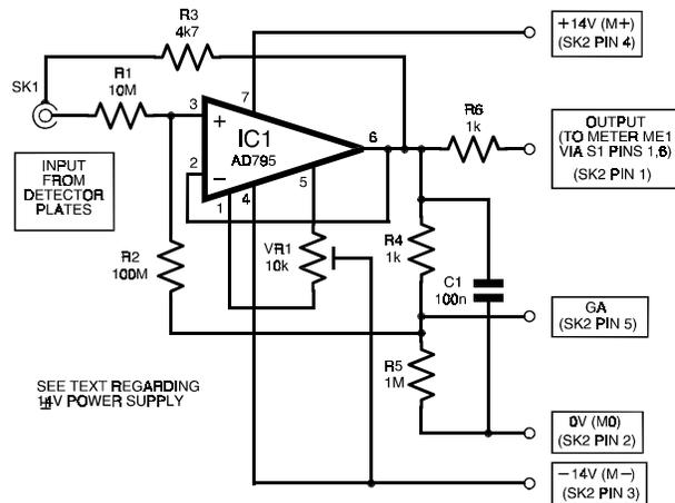
Fig.4. Circuit diagram for the meter interface buffer.
