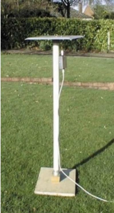
*The author's prototype single-plate atmospheric detection platform.*
