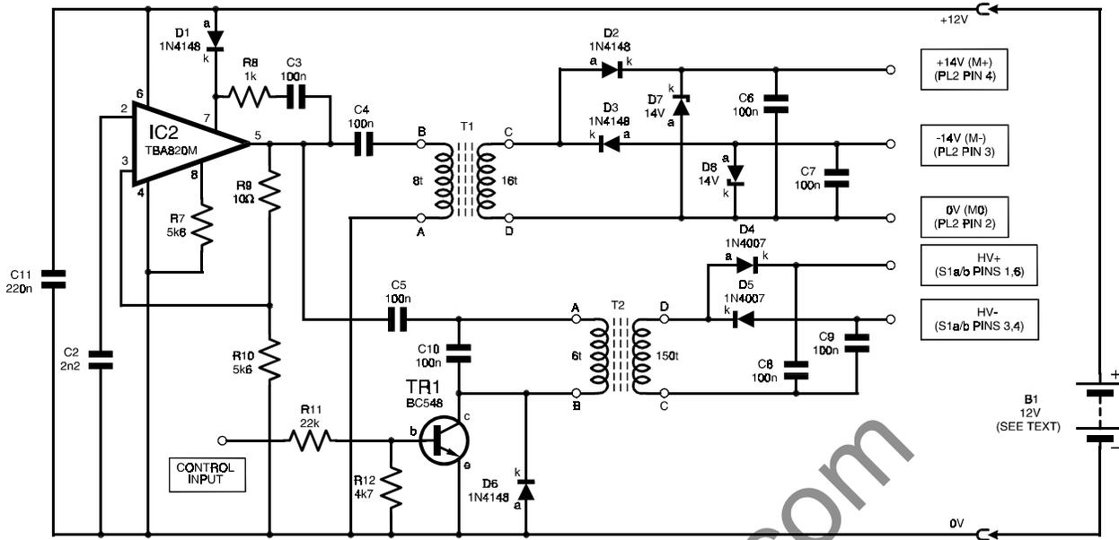
Fig.5. Dual voltage power supply generation circuit diagram plus variable 300V supply.
