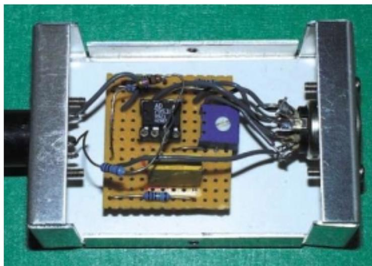
The meter interface board mounted in its case. A piece of card is placed between the board and bottom of case to prevent any "short circuits".
