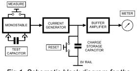
Fig.1. Schematic block diagram for the Low-Cost Capacitance Meter.
