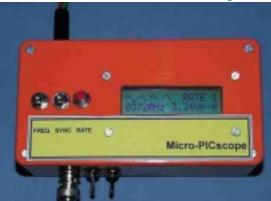
Completed Micro-PICscope showing general layout of display and controls.
