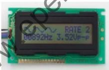
Close-up of typical screen display. There are three rates, the maximum counting frequency is about 17kHz.
