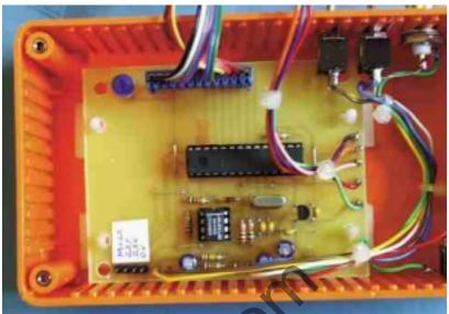
Completed circuit board mounted on self-adhesive plastic stand-off pillars.
