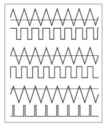
Fig.2. Example pulse width modulation (p.w.m.) waveforms.
