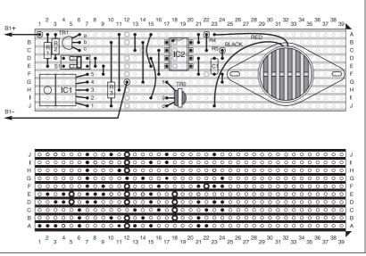
Fig.2. Fridge/Freezer Alarm stripboard component layout and details of breaks required in the underside copper tracks.
