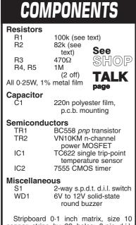
Stripboard 0.1 inch matrix, size 10 copper strips by 39 holes; 8-pin d.i.l. socket; AA size cells with holder – see text; battery clips, double-sided adhesive pad; multistrand connecting wire; 1mm solder pins (2 off); solder, etc.
