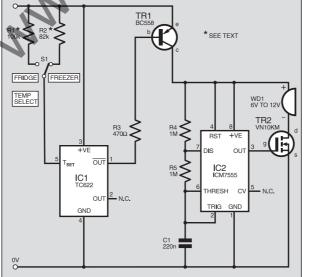
An intermittent tone is always much more noticeable than a continuous tone so the next stage in the circuit is an astable based on a 7555 timer (IC2). The values of the resistors R4 and R5 and the capacitor C1 are chosen to give a frequency of just over 2Hz. This produces an "urgent" rate of beeping that is easily heard from outside the freezer.
