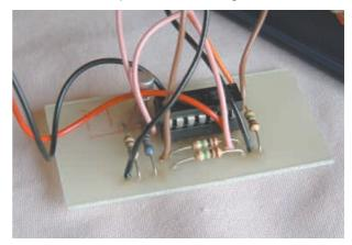
(Above) Completed circuit board removed from its case.
