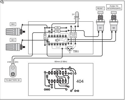
Fig.2. Printed circuit board component layout, off-board interwiring details and fullsize copper foil master for the Alarm System Fault Finder. The extra board width is to allow the p.c.b. to slot into the author's plastic box internal "guide rails".
