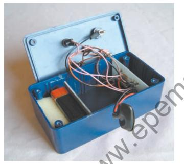
Prototype model showing the p.c.b. and battery compartment divider slotted into the case. The space between boards is to accommodate the lid-mounted components.
