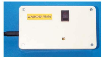
buzzer used. The internal 6V battery pack will provide several hundred operating hours and will probably give more than one year of service.
