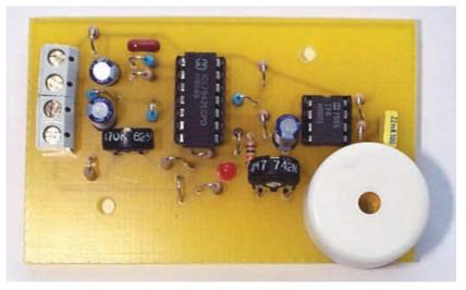
Component layout on the finished circuit board.
