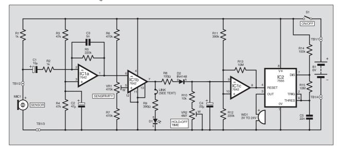
Fig.2. Complete circuit diagram for the Washing Ready Indicator. The battery pack B1 is made up of 4 x AA alkaline cells. Everyday Practical Electronics, May 2002
