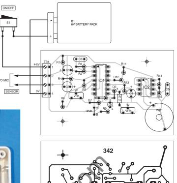
Positioning of components inside the plastic case.
