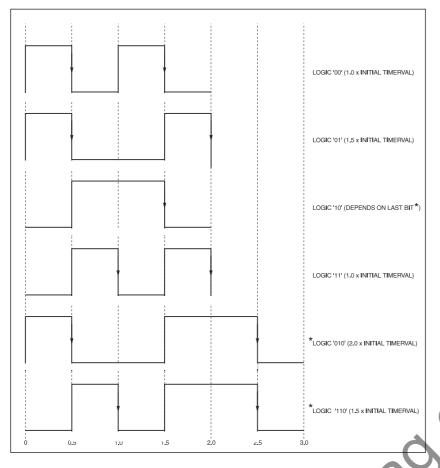
Fig.7. Example RC5 timing diagram.
