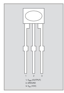
Fig.4. Pinouts for the IS1U60 sensor.
