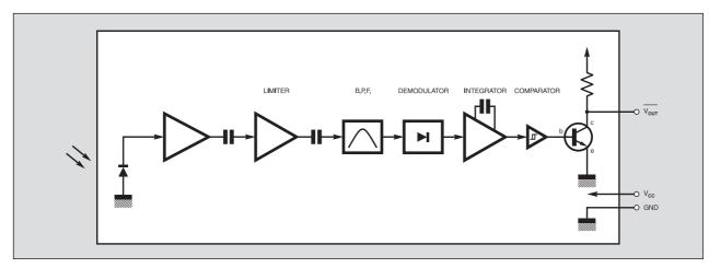
Fig.3. Block diagram for the IS1U60 remote control IR sensor.
