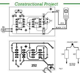
Fig.2. Printed circuit board component layout and (approximately) full size copper foil master pattern. Fig.3 (inset). How to make up R5 by wiring two resistors in series.
