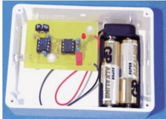
Completed unit showing positioning of the circuit board and the two-cell holder. Note the light dependent resistor (LDR) mounted in one side panel.
