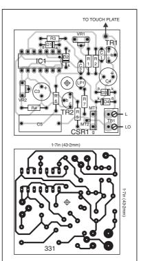
Fig.2. Printed circuit board component layout and full-size copper foil master. Note, a small "window" is cut in the centre of the p.c.b. for the neon light to shine through.
