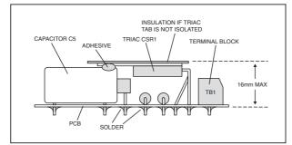
Fig.4. Suggested method of mounting the triac on the circuit board.
