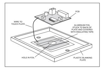
Fig.5. Suggested touch switch assembly.
