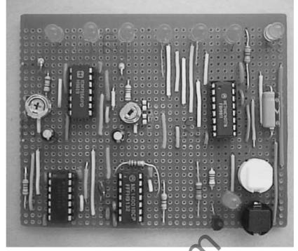
Steeplechase prototype circuit board.
