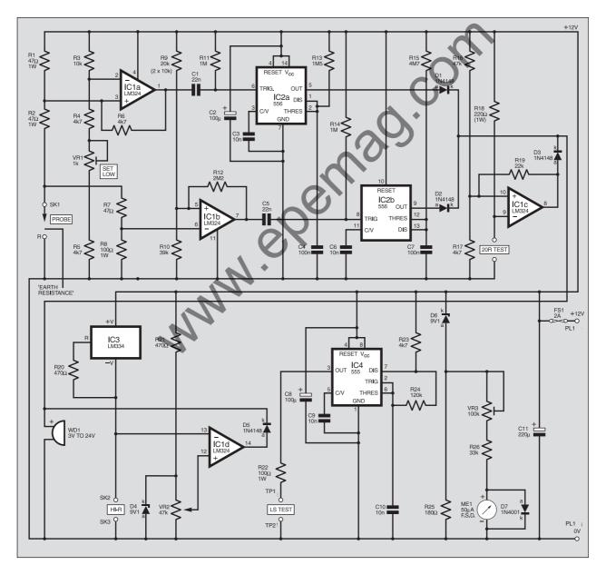
Fig.1. Complete circuit diagram for the Motorists' Buzz-Box. Note that some resistors must be rated at 1W. Everyday Practical Electronics, December 2000
