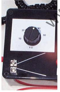
The "test" rails made from paper clips and the cardboard "resistance" scale.
