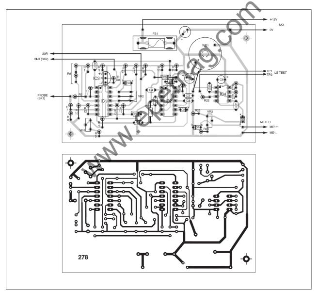
Flg.2. Printed circuit board topside component layout and full-size copper foil master for the Motorists' Buzz-Box.
