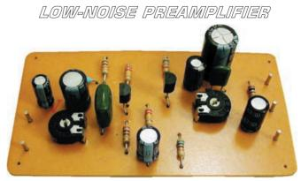
Completed p.c.b. for the Low-Noise Preamplifier.
