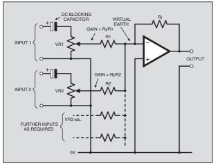
Fig.2. Adding extra inputs to the "virtual earth" mixer circuit.
