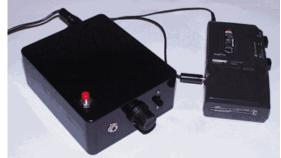
Completed Easy-Typist showing the additional pause-switch button on top of the case.
