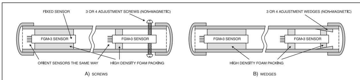
Fig.4. Alternative techniques for mounting the FGM-3 sensors, as used by Carl Moreland ([www.tthn.com/geotech](http://www.tthn.com/geotech)).
