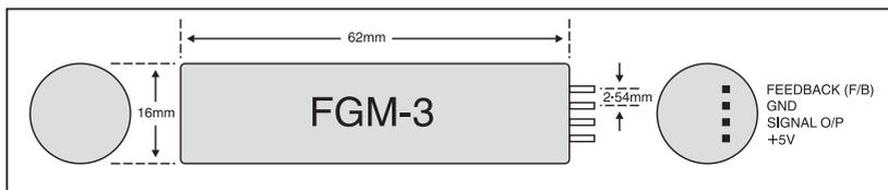
Fig.3. Details of the FGM-3 sensor module.
