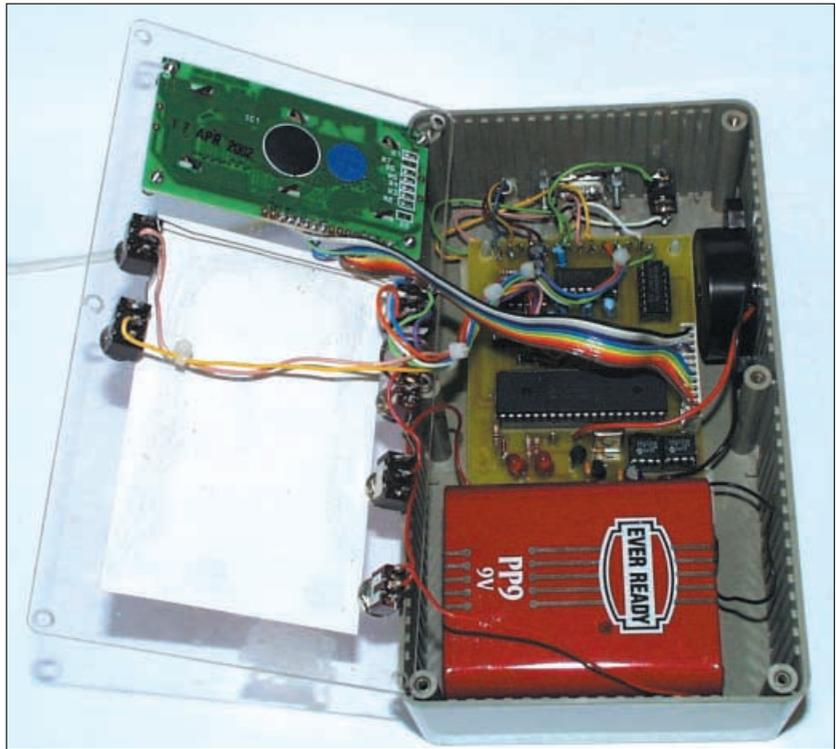
Observe the l.c.d. values. Very carefully adjust the precise orientation of the sensors until the two readings are as close to each other as you can achieve. There is always likely to be a difference, however, due to the individual characteristics of each sensor.
