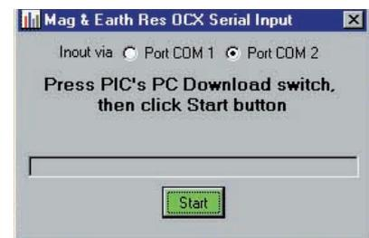
On receipt of each data block the PC and PIC again exchange "G" and "R" and another block is sent. This continues until the PIC recognises two zeroes in the data being extracted from the memories, or until the data in all memory locations has been sent. The PIC "knows" how many memories are installed and behaves accordingly.
