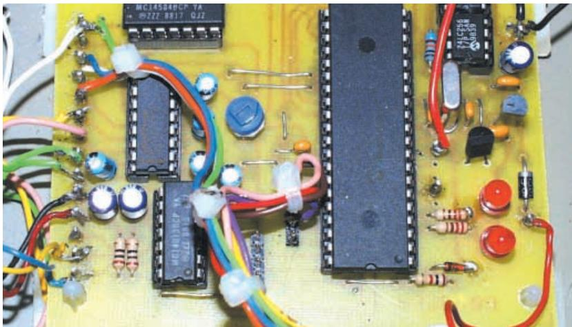
who wish to modify the published software for their own needs and then send to the PIC *in situ*. Diode D1 and resistor R3 prevent programming voltages adversely affecting the unit's 5V supply line.
